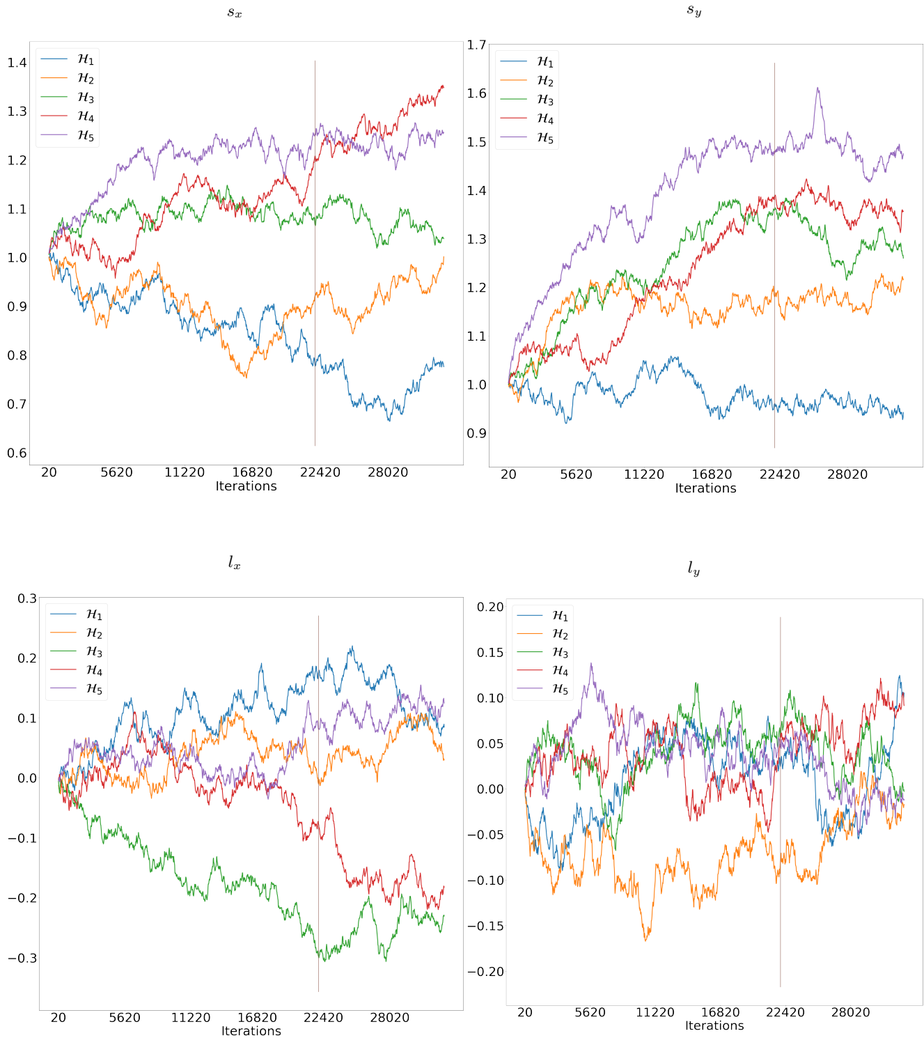
Figure A.4. Diversity in \mathcal{T} : We train |\mathcal{T}| = 5 initialized with \mathcal{H}_i = I . Homographies parameterized by s_x, s_y, l_x, l_y evolve as the training proceeds and tend to become diverse. Each homography is shown in different color. Even though we do not enforce any diversity, our approach learns diverse set of transformations. With these learned homographies, we achieve 79.5 AP@0.5 score for FoV adaptation task. The best score is achieved at iteration = 22k shown with the vertical line.
